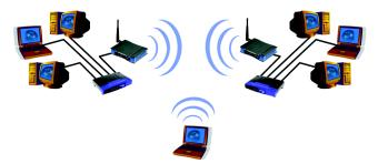
Figure 2-3: Network Using Wireless Bridging
